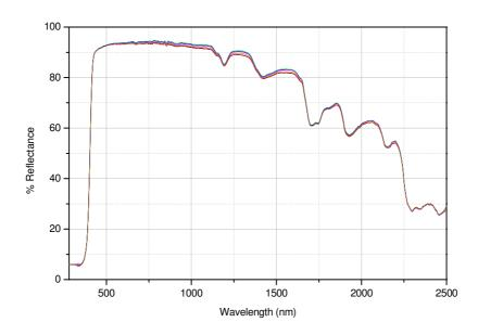
The result of solar reflectance of the test specimen referenced as **«QLR ONE»** is:
